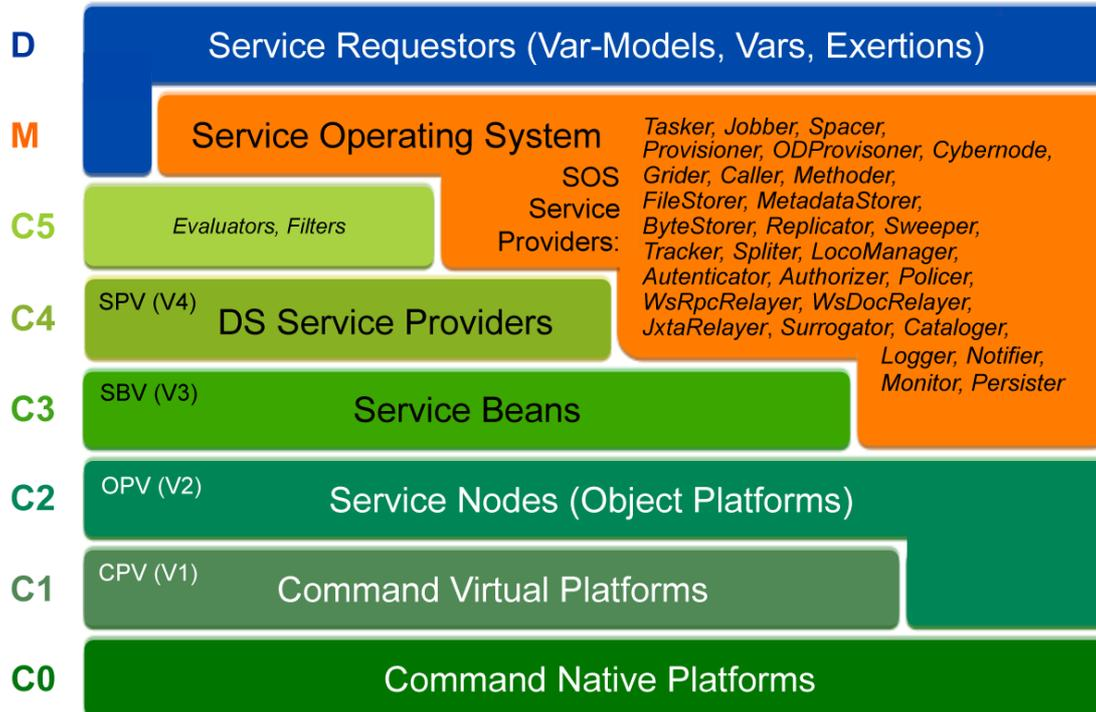
Figure 2. The SORCER layered architecture, where C0-C5 (carrier)—the metaprocessor with its service cloud at C4 and C3, platform cloud at C2 and C1, M (management)—SORCER operating system, D (domain)—service requestors; where V1-V4 stands virtualization of the corresponding layer.
