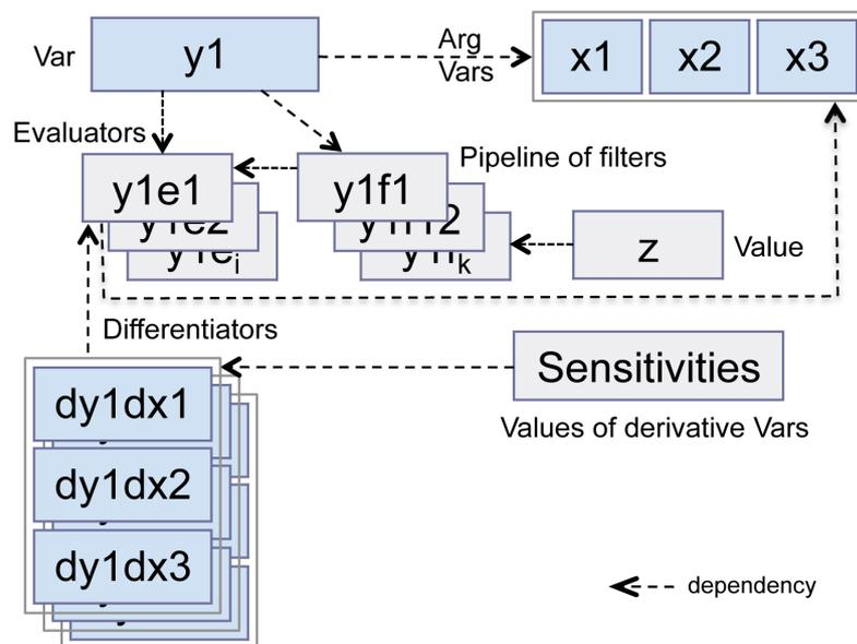
Figure 3. The var structure: value/evaluator/filter. Vars are indicated in blue color. The basic var  $y_1$ ,  $z=y_1(x_1, x_2, x_3)$ , depends on its argument vars and derivative vars.
